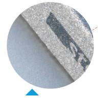
The Costa Stem system is manufactured from a titanium alloy Ti6AlNb (ISO 5832-11). The corundum-blasted surface has a roughness Ra of 4-6  $\mu m.$
